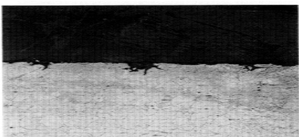
Pitting corrosion damage of Inconel 600
