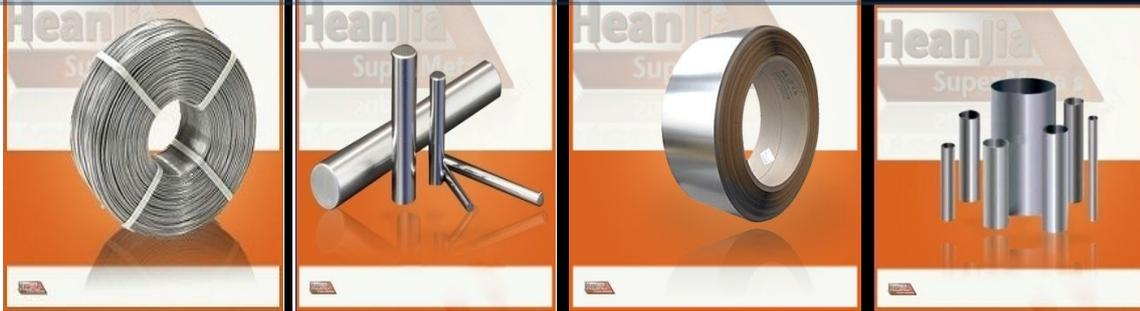
Nickel-Iron-Chromium alloy Incoloy 800 has fine strength and suitable resistance to oxidation and carburization at high temperatures. It offers elevated temperature performance in the petrochemical industry as it prevents the formation of embrittling sigma phase subsequent to prolonged use up to 1200oF or 649oC. Alloy 800 is used in the industrial incinerators, heat processing equipments, chemical processing industries etc.
